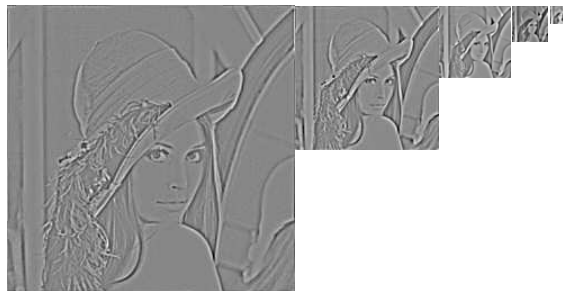
(b) The Laplacian pyramid
