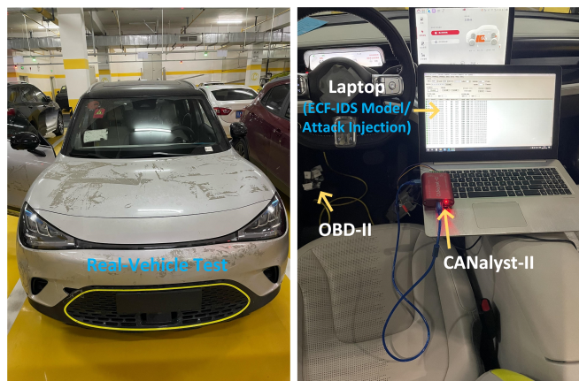
Fig. 16. Real Vehicle Test of ECF-IDS Model
